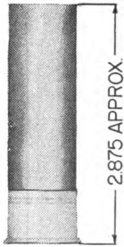
FIGURE 16.—Shell, shotgun, 10-gage, blank (8 grains black powder with dry felt wads).
